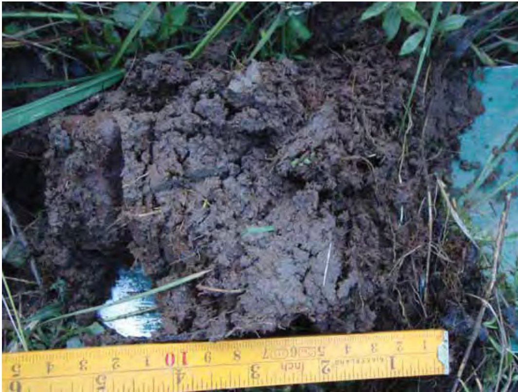
Figure 5: Soil profile at site Wet 3 located in Marsh 5 on the southern extent of the project area. Undecomposed roots are visible throughout the matrix. Note the large stone at 12 cm. Sand/gravel/stone layer existed below 15cm.
