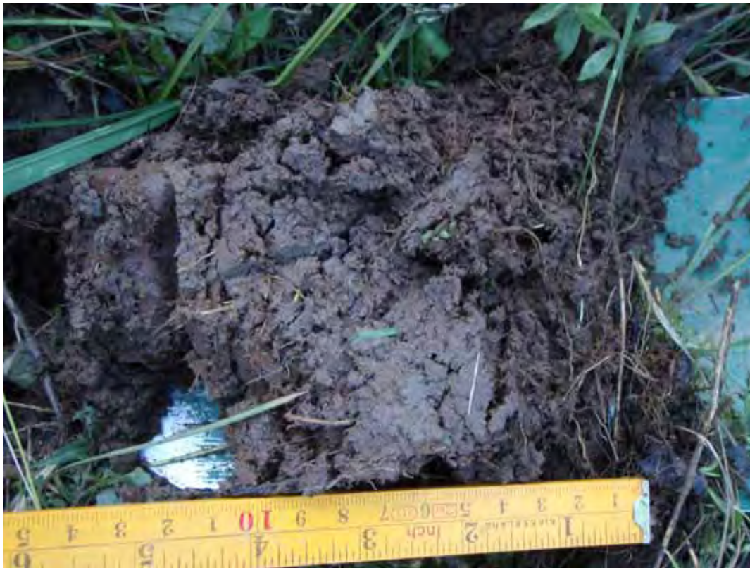
Figure 7: Soil profile at site Wet 3 located in Marsh 5 on the southern extent of the project area. Undecomposed roots are visible throughout the matrix. Note the large stone at 12 cm. Sand/gravel/stone layer existed below 15cm.
